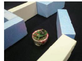
Fig. 8 Stationary Epuck observing landmarks
