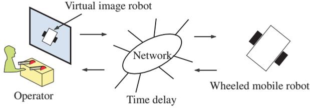
Fig. 2. Bilateral Teleoperation using Virtual Image Robot
